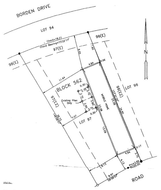
Unless atherwise specified, the dimensions shown related to distance found from property boundaries to structure walls only at the date of survey. There are no measurements pertaining to footing, roofing, etc. This plan is for the protection of the Mortgagee only and is not to be used for the location of the property lines. We accept no responsibility for the unauthorized use.
